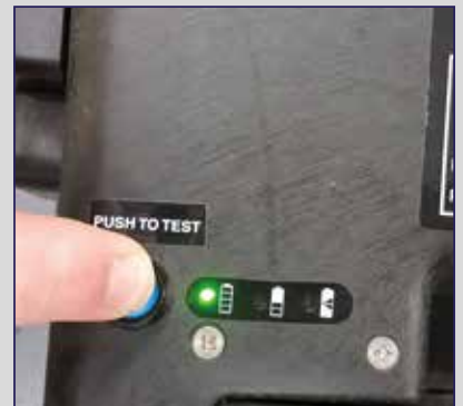
Battery status indicator Green | Amber | Red
